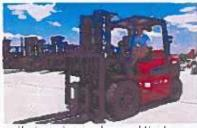
Working in containers enroduces special implict constraints. The available 67' reduced height overhead guard is purpose suit for this law height application.
