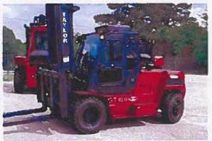
of Capacity: 18,000-lbs (8,165 kg) Load Center: 24-in (510 mm)
